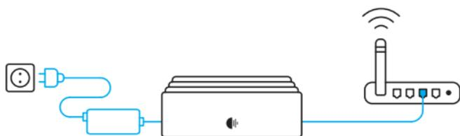
**Nucleus:** Connect the power supply to Nucleus and plug it in. Use an ethernet cable to connect Nucleus to your router or switch.
