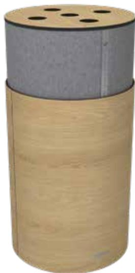
**Vari Bass Ultra** is designed for use in any Hi-Fi room. Made from wood and high-density acoustic foam, the bass trap can be tuned between 50Hz-100Hz by simply rotating its wooden top (which has a series of resonant pots) until the problem disappears. A scale is included to show the exact frequencies on which the Vari Bass Ultra is acting. The unit's stand-alone structure enables it to be repositioned as required and used in different rooms.
